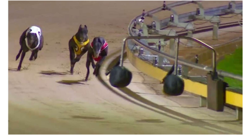
Traditional Victorian steel post & lure rail system with irrigation sprays on safety rail
