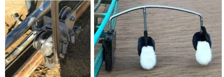
Traditional cable and roller lure system in operation at most tracks across Victoria
