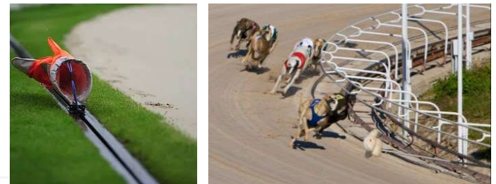
UK lure operated from an underground rail and cable on the outside
